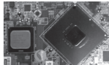
D520PT with US15WPT supports wide temperature of -40°C ~ +70°C
