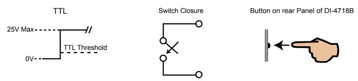
The built-in remote control jack located on the front panel of the DI-4718B accepts a standard 3.5mm stereo phone plug (provided) and provides access to remote events and stop/start remote recording control features. The Remote Control Feature can be used in Stand-alone mode or when using WinDaq Acquisition software.
