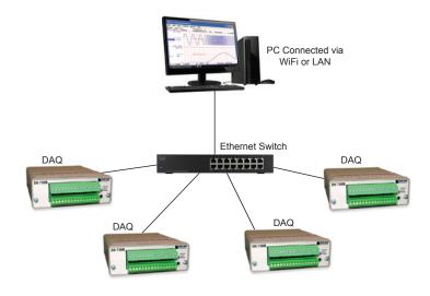
Max cable length: 100 meters Sample rate: Up to 5 kHz per channel DAQ: Any Ethernet-enabled DI-4718B
