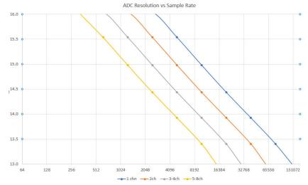
ADC resolution (R) is a function of selected sample rate per channel (F), and the number of enabled analog channels (C):
