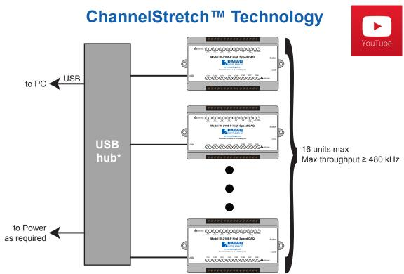
\*DATAQ Instruments 7-port USB hub (part number 2000310). Cascade for a higher port count.
