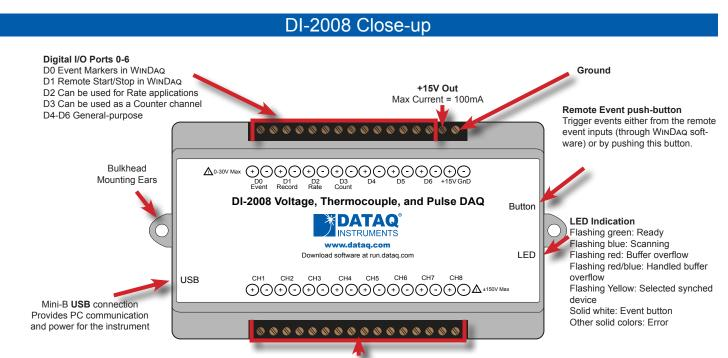
Analog In Channels 1-8 (programmable Voltage or Thermocouple) Voltage Ranges:  $\pm 10$ , 25, 50, 100, 250, 500 mV;  $\pm 1$ , 2.5, 5, 10, 25, 50 V; Thermocouple Types: J, K, T, B, R, S, E, N
