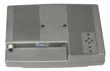
Rear view of the Datalux 12.1" monitor shows locking power connector and communications connector, VGA connector and USB connector. When in use, the control panel would normally be covered and sealed. Standard 75mm VESA mounting holes are supplied along with holes for Datalux locking clamp. All connectors and cables exit from a bottom recess on the back of the display.
