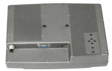
Rear view of the Datalux 10.4" monitor shows locking power connector and communications connector, VGA connector and USB connector. When in use, the control panel would normally be covered and sealed. Standard 75mm VESA mounting holes are supplied along with holes for Datalux locking clamp. All connectors and cables exit from a bottom recess on the back of the display.
