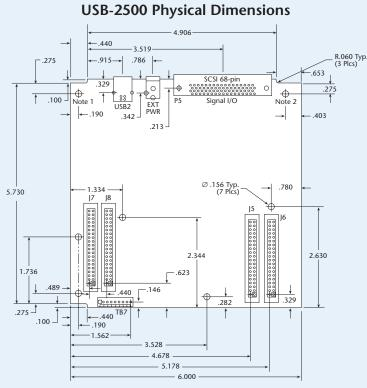
general, all standoffs should be used to mount the board to a metal frame
