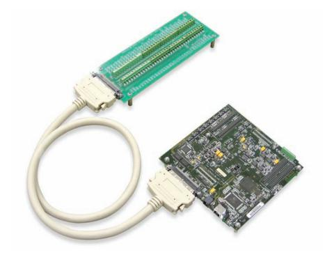
USB-2527 attached to a TB-100 screw-terminal board
