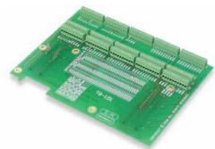
TB-101, termination board with screw terminals, provides access to all USB-2500 Series I/O. The TB-101 mounts directly onto the board with included hardware.
