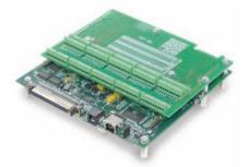
USB-2527 with TB-101 screw-terminal board attached
