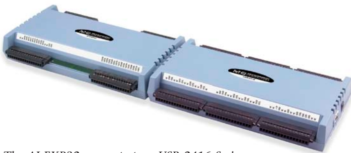
The AI-EXP32 connects to a USB-2416 Series device with included hardware
