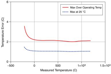
Temperature error of J type thermocouple
