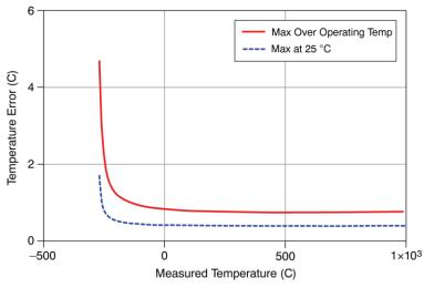
Temperature error of E type thermocouple
