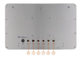
1. Backlight on/off 6. 1 x RS-232/422/485 (default RS-232) 2. Brightness adjust +/-7. 1 x RS-232/422/485 (default RS-232)
