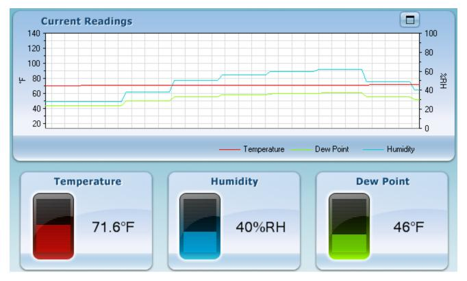
The EL-USB-RT software clearly displays real-time temperature, humidity and dew point in real time on the host PC's display.
