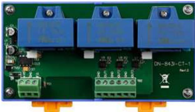
DN-843I-CT-1 is a current input sensor, it have the maximum input range  $\pm 1$  A to  $\pm 1.6$  V. If you combine analog input module such as I-7017 and I-87017 etc. You can monitor or measure the Current.
