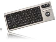
The DBL-810-TB features integrated green LED backlighting for use in low-light e nvironments, and is sealed to NEMA 4X specifications.
