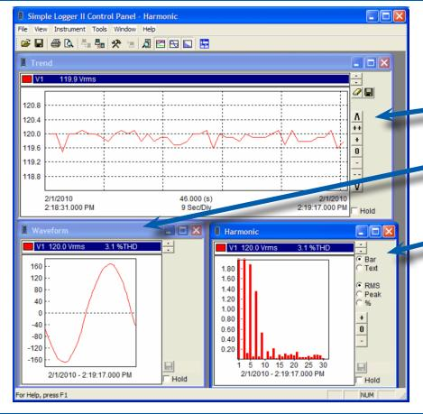
The **Trend** Display window shows measurement (sample points) over a time period.
