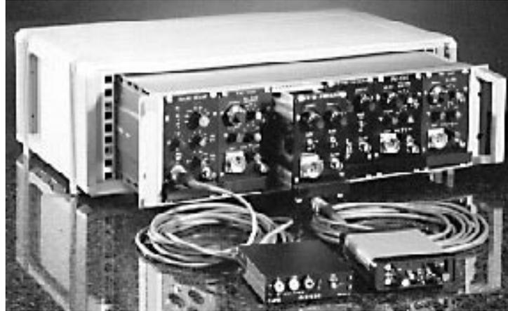
Desktop enclosure (DTE-1000) housing CC-1000 amplifier cage.
