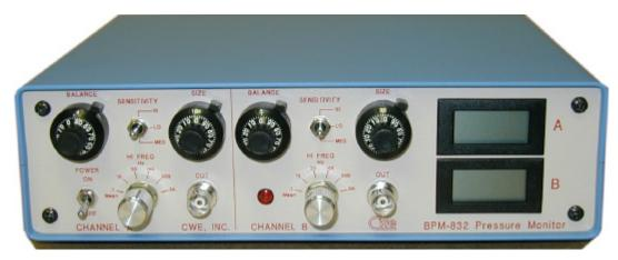
The BPM-832 Pressure Monitor provides two independent amplifiers for use with bridge-type transducers, including pressure, force, and acceleration. Each channel includes a high-gain preamplifier, low-pass filtering, adjustable DC balancing, and a digital readout.
