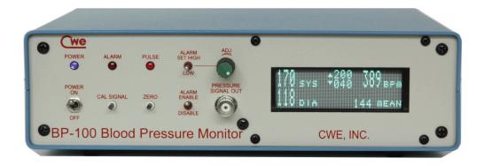
The **BP-100 Blood Pressure Monitor** is an accurate, easy-to-use instrument for measuring direct blood pressure (BP) from small animals. It is designed to operate using standard, widely available clinical-type BP transducers (included with unit). In addition, miniature catheter-tip transducers are available for high-resolution intra-arterial BP measurements. The standard *systolic*, *diastolic*, and *mean* pressures are reported, along with *heart rate* (HR).
