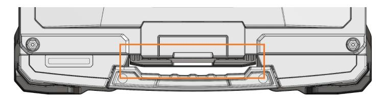
6) For theft deterrence, secure computer by locking Docking Station with supplied key (Hardware Kit item 2).
