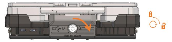
2) Unlatch computer from Docking Station by pushing on the Release Handle in the direction shown below. Once unlatched the computer will rise above the front latch hooks.
