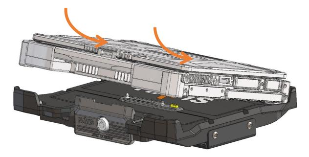
4) Lower front of computer onto Docking Station, ensuring computer properly aligns with the front fence on the Docking Station. Apply downward pressure to the front of computer, until Front Hooks on Docking Station snap into place and secure the computer. Ensure Front Hooks are fully engaged by trying to pull up on the laptops handle.
