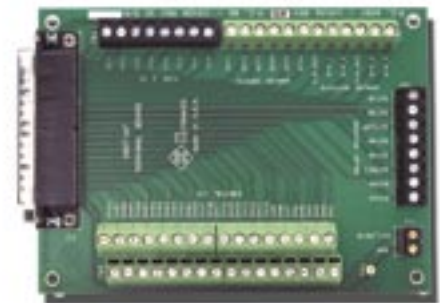
4807/2307 Terminal Board Assembly
