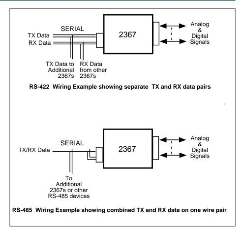
Figure 2 RS-422 and RS-485 Wiring Examples
