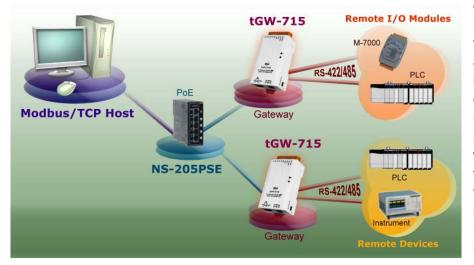
communicate with serial Modbus RTU/ASCII devices through an Ethernet network, and eliminates the cable length limitation of legacy communication devices. The module can be used to create a pair-connection application (as well as serial-bridge or serialtunnel application), and can then route data over TCP/IP between two serial Modbus RTU/ASCII devices, which is useful when connecting mainframe computers, servers
