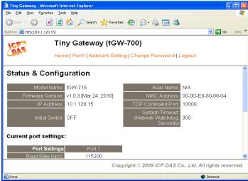
The tGW-700 module features a powerful 32-bit MCU to enable efficient handling of network traffic, and also has a built-in web server that provides an intuitive web management interface that allows users to modify the configuration of the module, including the DHCP/Static IP, the gateway/mask settings and the serial port settings.
