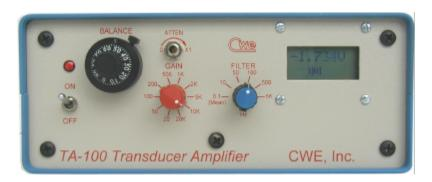
The TA-100 is a compact, stand-alone amplifier for use with all DC-bridge type transducers. Compatible transducers include blood or air pressure, strain gages, force transducer, and accelerometers. A built-in LCD display shows the current measurement as well as a fast-response bar-graph for easy visualization of a changing signal. A standard serial port allows remote data collection using any simple terminal software.
